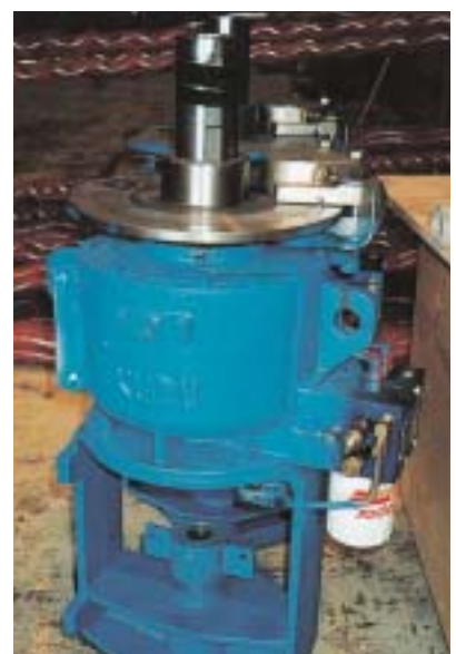
2 - Drive head with back spin brake (Kudu)
